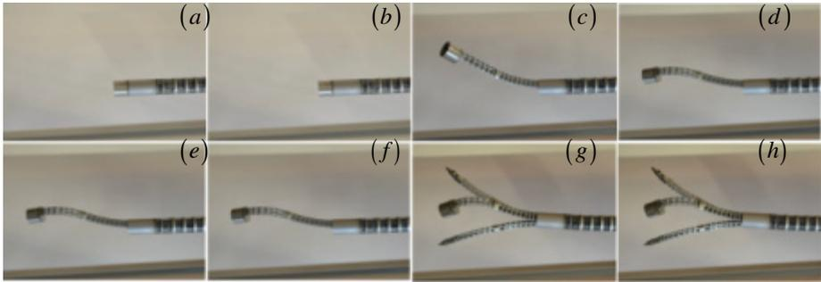
**Fig. 10.** Deployment of the endoscopic robotic device
