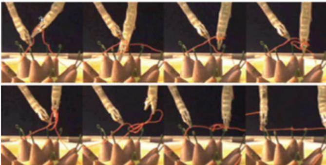
**Fig. 8.** Knot tying was achieved by continuum robots with similar structures as in [15]
