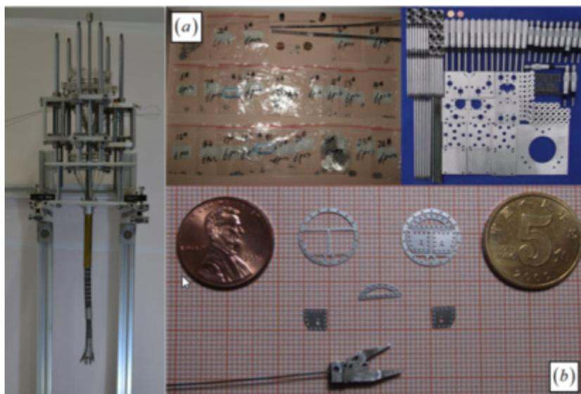
**Fig. 9.** The endoscopic continuum robot assembled with the manual actuation unit: (a) all the components of the endoscopic continuum robots and (b) a few components with respect to US and Chinese coins on a piece of graph paper
