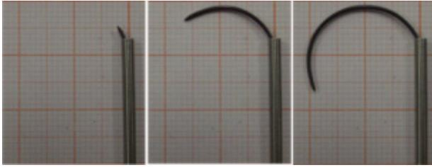
**Fig. 5.** A  $\text{\O}0.69\text{mm}$  suture made from pre-curved NiTi alloy: it bends back to its original circular shape after released from a straight rigid housing. The suture's radius is about 9mm. Thinnest grids in the background are 1mm x 1mm.
