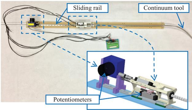
Fig. 1. Design of the continuum tool for shape sensing
