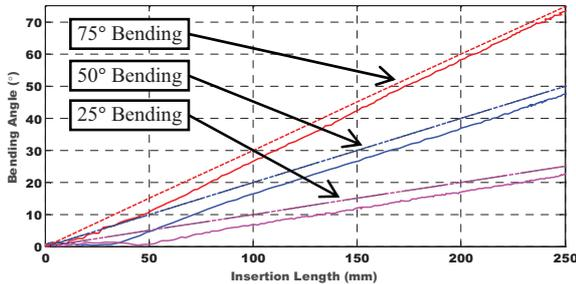
Fig. 6. Results of the tool calibration on the bending angles: dashed lines for the reference values and solid lines for the sensed values
