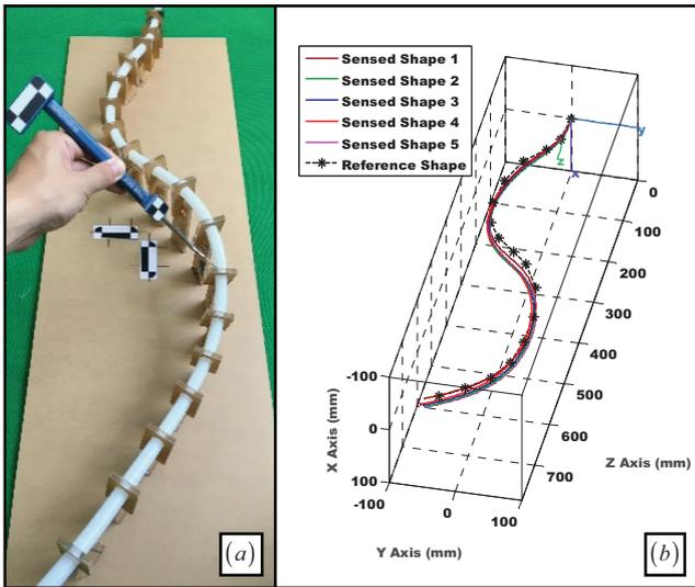
Fig. 8. Experimental validation: (a) the spatial lumen for shape sensing, and (b) the sensed shapes
