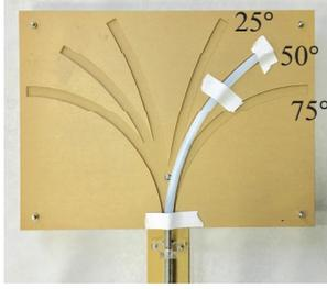
Fig. 5. PTFE lumens with known shapes for the tool calibration
