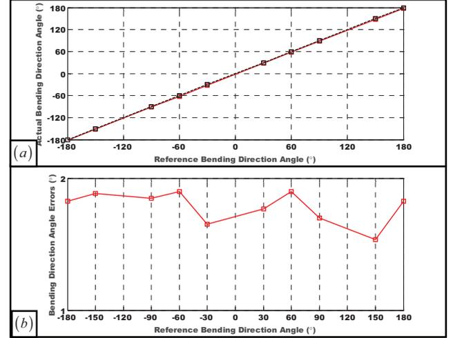
Fig. 7. Results of the tool calibration: (a) bending direction angles, and (b) errors
