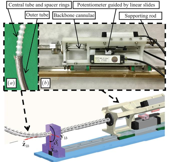
Fig. 4. System description of the insertable continuum tool: (a) the insertable continuum portion, and (b) the 3D printed sliding base
