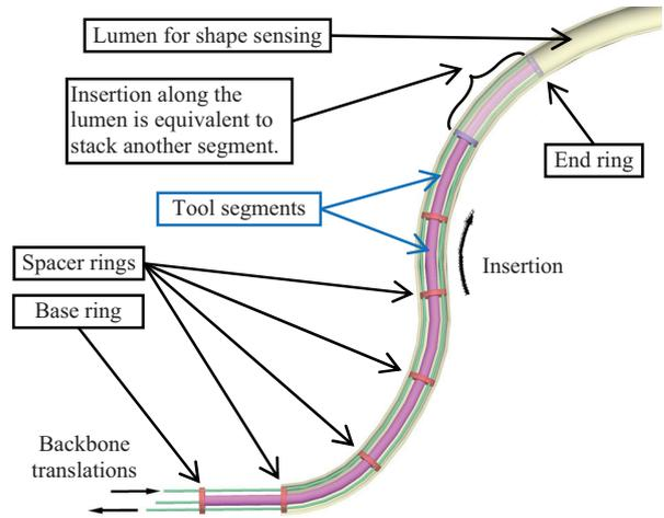
Fig. 2. Working principle of the continuum tool for shape sensing
