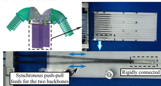
Fig. 5. The transmission unit
