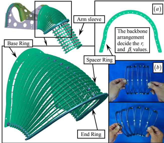
Fig. 4. The continuum shoulder brace: (a) the backbones arrangement, (b) the riveted spacer rings
