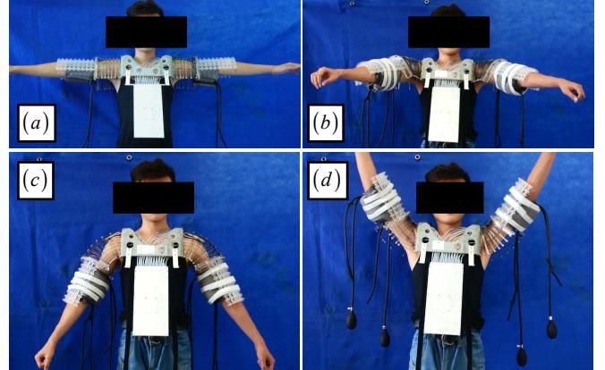
Fig. 8. Bilateral motions of a human subject: (a) before the arms were attached, (b) to (d) various bilateral movements
