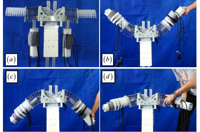
Fig. 7. Bilateral motions of the mockup patient using the exoskeleton: (a) before the arms were attached, (b) to (d) various bilateral movements
