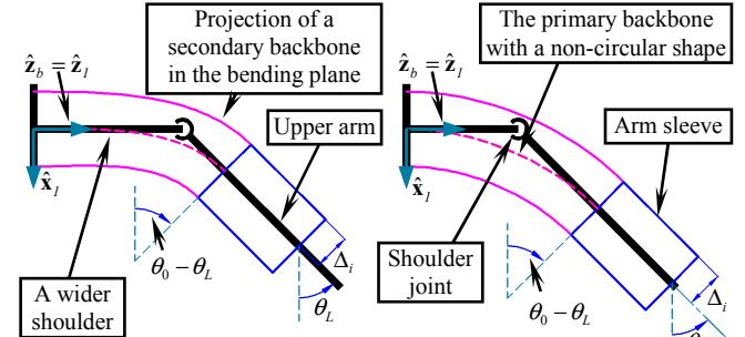
Fig. 3. A schematic diagram for the shoulder exoskeleton while worn on patients with different shoulder widths
