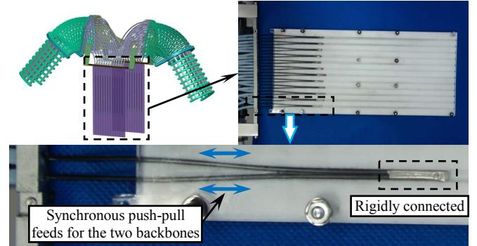
Fig. 5. The transmission unit
