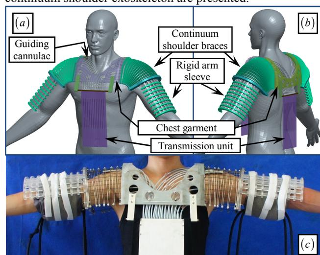
Fig. 1. The compliant continuum shoulder exoskeleton for self-provided bilateral rehabilitation: (a) the front view, (b) the back view, and (c) the prototype worn on a human subject
