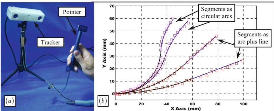
Fig. 9. Shape identification of the tool's continuum arm
