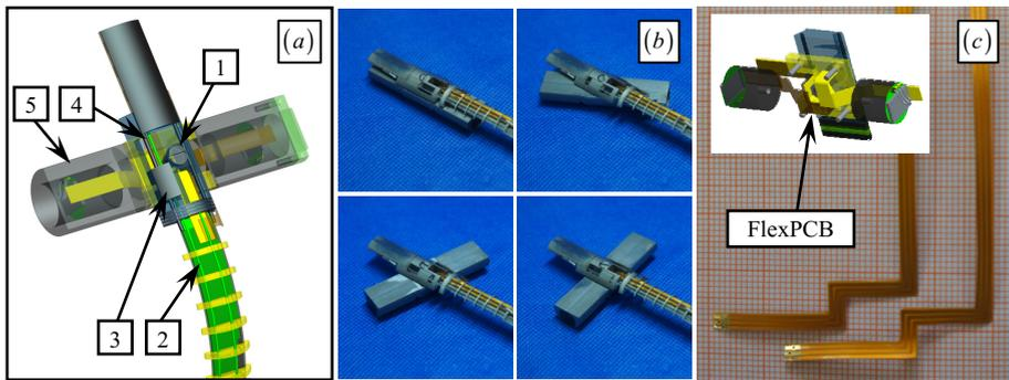
**Fig. 4.** The pivoting mechanism for the camera head: (a.1) pivoting screw, (a.2) actuation rod, (a.3) actuation block, (a.4) pin guide, (a.5) camera head, (b) the motion sequence, and (c) arrangement of the FlexPCB
