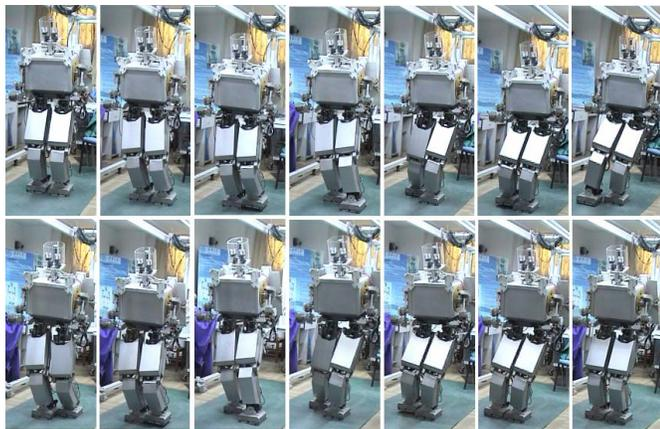
Fig.12 Walking on flat ground (Sequence photographs: 2.0 [sec/frame])
