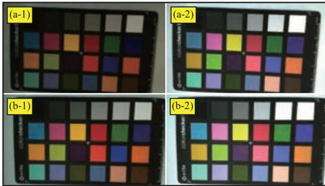
Figure 6. Laparoscopic images of the X-Rite ColorChecker Classic Mini color chart (a-1)(b-1) before correction, and (a-2)(b-2) after correction
