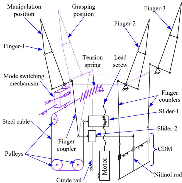
Fig. 2. Actuation strategy of the gripper.
