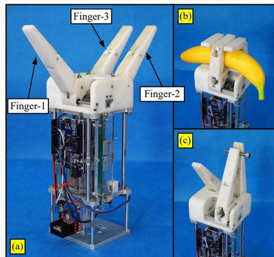
Fig. 1. The proposed gripper: (a) an overview, (b) the gripper in the grasping mode and (c) in the manipulation mode.
