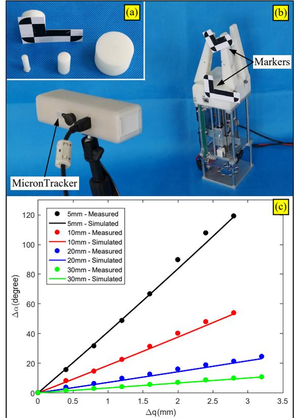
Fig. 9. Manipulation experiments: (a) cylindrical objects, (b) experimental setup, (c) simulated and measured results of rolling cylindrical objects
