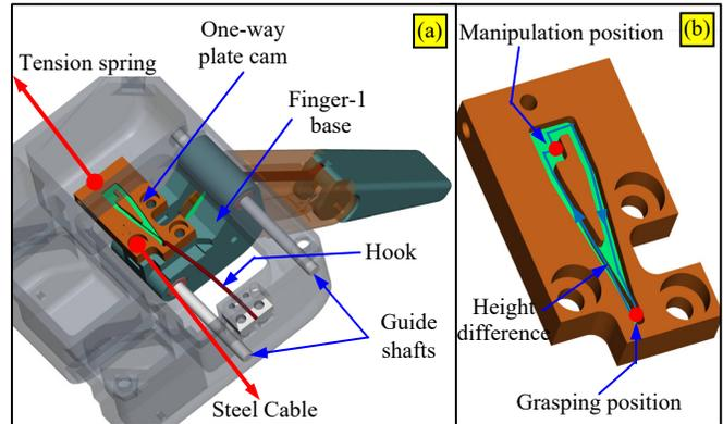
Fig. 5. The working mode switching mechanism: (a) schematic of the mechanism and (b) detail of the one-way plate cam
