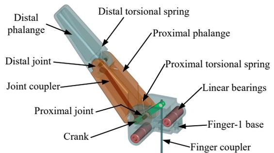
Fig. 3. Design of the fingers: (a) index finger and (b) thumb
