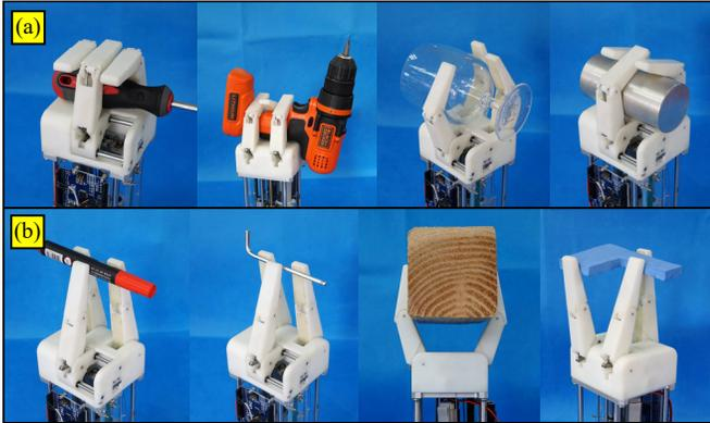
Fig. 8. Grasping experiments: (a) power grasps and (b) pinches
