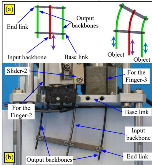
Fig. 4. The CDM: (a) schematic and (b) the implementation in the gripper
