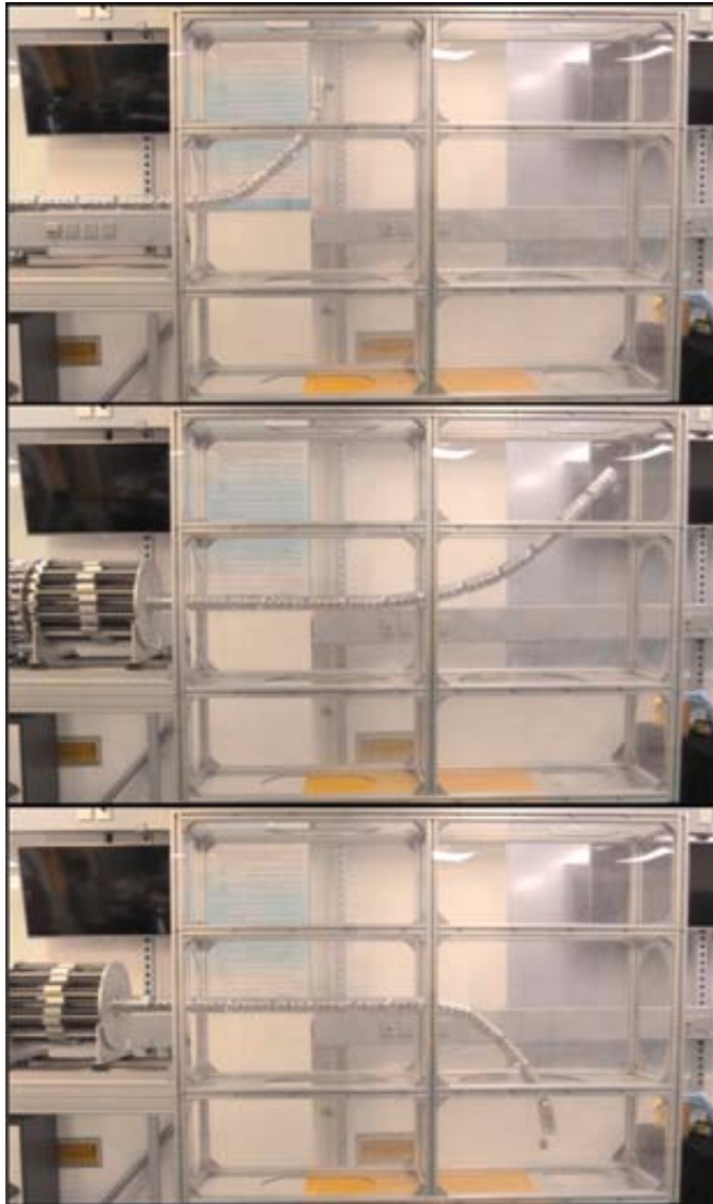
Fig. 15. Inspections to different cavities of a center wing tank model.
