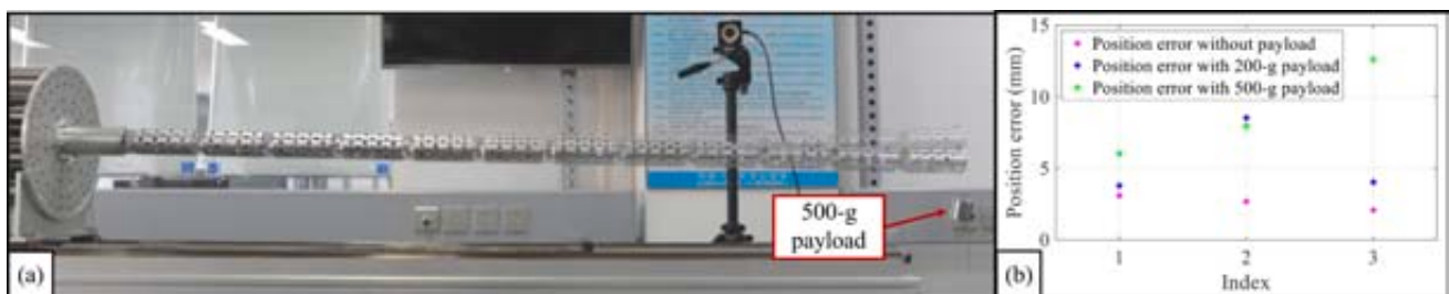
Fig. 13. Payload capability test: (a) the straight manipulator deflected by a 500-g weight without the closed-loop controller; (b) tip position errors under different payload conditions.
