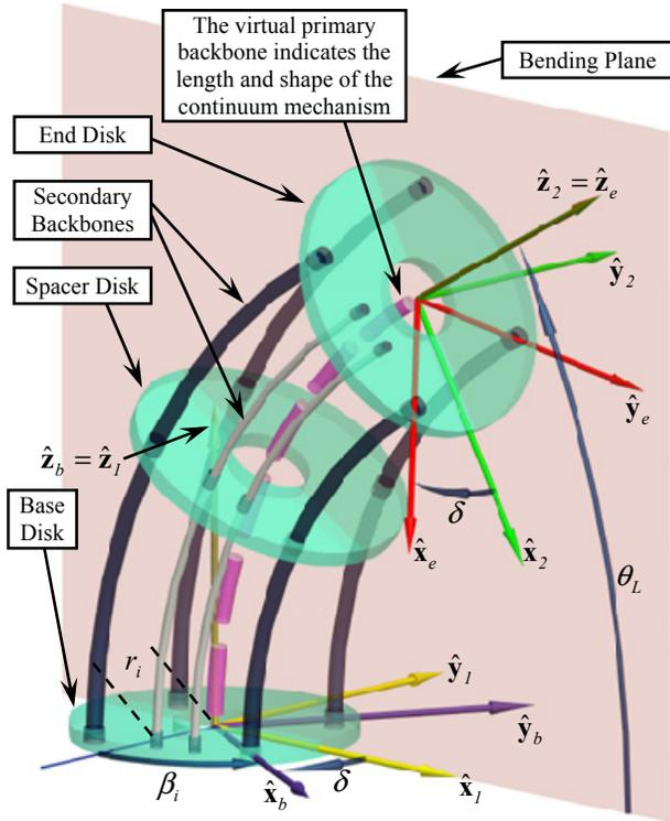
Fig. 5. Nomenclature and coordinates of the continuum mechanism
