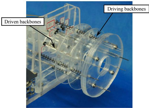
Fig. 6. The continuum mechanism for the synergy implementation
