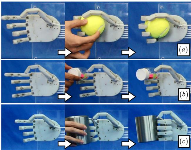
Fig. 9. Grasping poses realized using the  $g_{1i}$  and  $g_{2i}$  values from Table I: (a) a tennis ball, (b) a pill jar, (c) a mug
